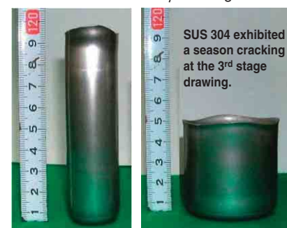
NSSC 304JS Seven-stage drawings (drawing ratio: 4.4) SUS 304 Two-stage drawings (drawing ratio: 2.2)
