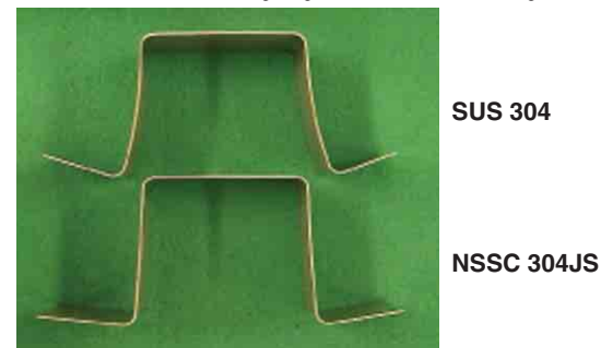
(NSSC 304JS exhibits only a minimal spring back after press.)
